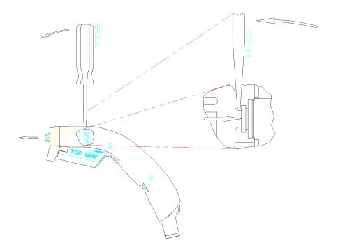
If the filter does not release, grasp the nozzle and rotate the filter as far as it will easily turn. Insert screwdriver and use gentle "prying" motion to free lock collar. Be very careful not to damage the chassis of Top Gun while using this procedure to replace the filter.
